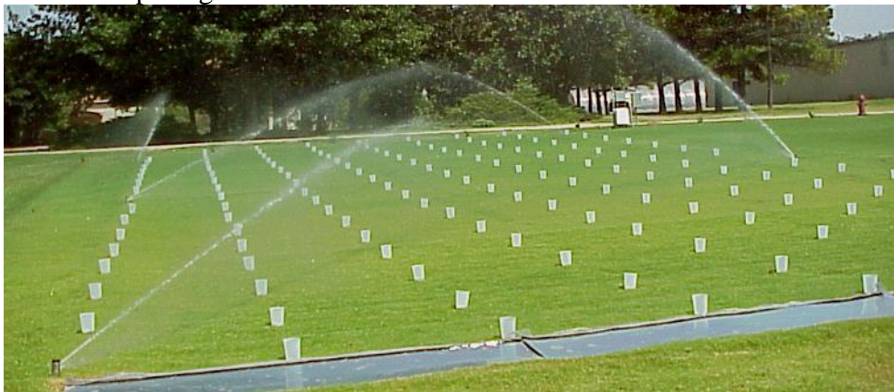
Figure Sprinkler evaluation in the field
